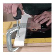
Place the right side edge of the stock against the in feed side of the fence.
