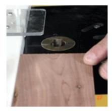
If the router bit still lines up with your centre guess mark, then you have found the centre of your stock. If your centre guess mark is wrong use your fine adjusting tool (hammer) to tap the fence in or out so it is exactly on the centre of the stock.
