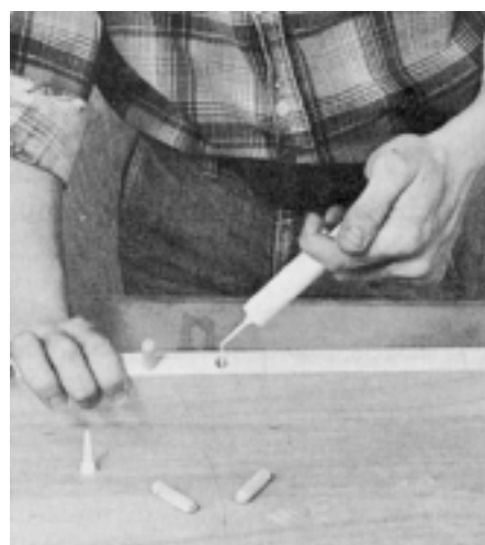
Figure 3. A glue injector is used for reaching small holes, cracks and tiny gluing surfaces.
