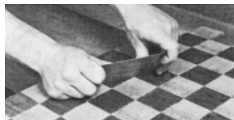
Figure 4. A cabinet scraper can be used to knock off glue beads.
