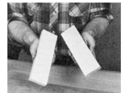
Figure 1. To get an even glue spread, apply glue to one surface, rub the two mating surfaces together in a circular motion, then check to be sure the glue has spread over the entire gluing surface.
