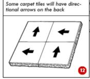
Check the manufacturer's instructions for the correct way to lay the tiles - some have arrows on the back, which show the direction in which each tile is to be laid (12). It's important to follow the arrows as, with plain tiles, it is this which gives the 'chequerboard' effect.
