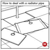
Where there is a radiator pipe, cut a slit from the back edge of the tile to the pipe position and then cut a circle out for the pipe. When the tile is laid, the slit will not be visible (10).
