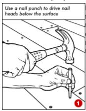
If you have chipboard floors which are smooth and level, you can lay tiles directly on top. Remove any protruding tacks or nails or drive their heads below the surface using a hammer and nail punch (1); drive any screws just below the surface. Any loose boards should be refixed - use screws in upstairs rooms as hammering could damage the ceiling below.
