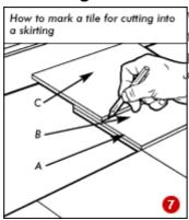
When cutting into a skirting (7), lay the tile to be cut (B) directly on to the last full tile in the row (A). Now place a third tile (C) on top and press its edge against the skirting. Using a pencil or biro, mark the other edge of tile C on to tile B.
