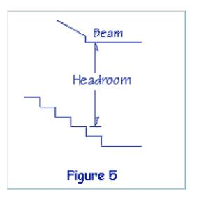
the stairs. The minimum headroom under a beam or joist is 1.95 m.(76 7/8"). Now that we have determined our rise and run and checked for adequate headroom, we can cut the stringers. (For more info on stringers see How to Cut Stair Stringers.)
