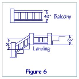
comfortable height. At a landing, the handrail should be 36" high and at a balcony edge should be 42" high. These measurements are for single dwelling residential construction (one family house).
