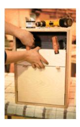
A consistent reveal is key to the crisp feel of the piece. The shims shouldn't bow the cabinet sides out at all, but should fit snugly to ensure that the drawer front is centred and that the reveal is even on both sides.
