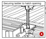
The screws used to secure the ladder fixings to the top of the trimmer may be quite large (4). Do not attempt to drive them in without first drilling pilot holes into the wood.
