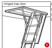
A good solution is a permanently fitted loft ladder that is hinged from a trap door opening (1) and can be folded up and kept out of the way in the roof space. Some ladders come complete with the hatch cover, frame and fittings.
