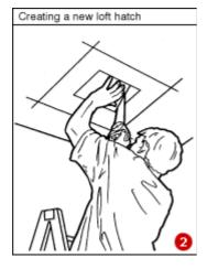
Mark out the square for the hatch opening (2). Using a general purpose saw cut an inspection hole between two joists within the marked area, large enough to accommodate your head and the trailing light. This will allow you to inspect the area for hazards and space requirements.
