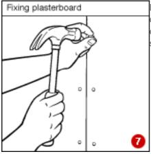
Drive nails up each edge (7) and into any central stud - you do not need to nail into the noggins. The nails should be driven until they just 'dimple' the surface - do not drive them so far that they break the paper.
