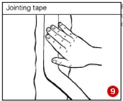
Position the tape over the joint, running the knife firmly down it to bed the tape in, squeezing out excess joint compound and air (9).
