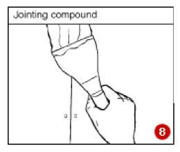
To join tapered-edge plasterboard, mix up clean plasterboard jointing compound in a clean bucket and press into joint with a filling knife (8).
