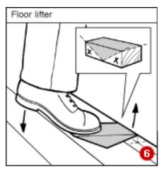
Lift it off the floor, using a 'floor lifter' (6) or a flat lever over a block of wood, so that it is tight up against the ceiling. Nail the board in place using 32mm plasterboard nails, 10mm from the bound edges and 12mm from the cut edges and spaced every 150mm.
