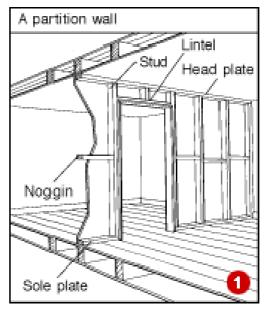
The framework of a partition wall has four main components (1):
