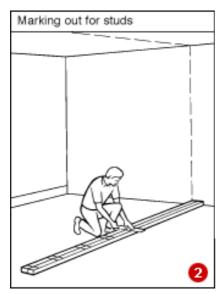
Cut the sole and head plates to length (remembering to allow for the doorway on the sole plate) and lay the pieces side by side to mark out the positions of the vertical studs (2). The width of the door opening is the width of the door + 6mm + twice the actual thickness of the door-lining material. There should be a full stud either side of the doorway (and a short stud in the centre): work outwards from these two studs to mark the remainder.
