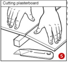
If necessary, cut the tapered-edge (T/E) plasterboard to 12mm (1/2in) less than the floor-to-ceiling height, using a trimming knife to score the surface and snapping the board over an edge (5). Remove the paper burr from the cut edge with fine sandpaper.
