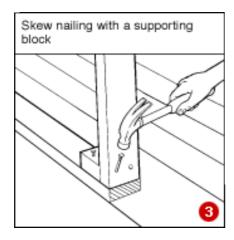
Fit the door studs next, cutting them to length to fit exactly between the sole plate and the head plate, then 'skew' nail them into position with nails driven at an angle through the end of the stud into the sole and head plate (3). Check (with a spirit level or plumbline) that the door studs are vertical and (with a tape measure) that they are correctly spaced before nailing them in position.
