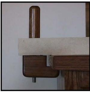
The through rod is 1/2" all thread and a nut is recessed into the bottom of the clamp block. The handle has about 1 1/2" of the all thread passing into it with a hole drilled horizontally through the handle and all thread. A pin is then inserted into the hole and glued in place - this keeps the handle from spinning on the all thread.
