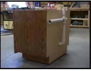
The next step is to provide piping for the suction from the fence and finally to the vacuum. In the picture (left), the sanitary 4-way tee has to be used because the turns are curved in the direction of the suction out, making it easy for
