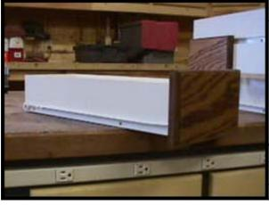
The type of drawer system you use is entirely up to you. I used drawer slides from *Blum* but since there are so many manufacturers of these things it's really difficult to address making drawers. I made mine with simple butt joints, stapled together. They are 18" long and 1 1/16" narrower than the drawer opening in the face
