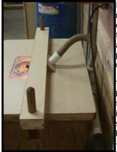
It would do no good to have debris remaining near the fence when it's so easy to provide for dust collection at that location too. The tee in the system allows you to extend another piece of pipe up near the tabletop so that a hose can connect the fence into the system.
