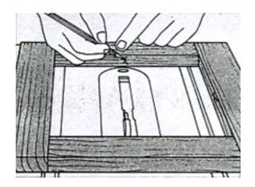
STEP 1: Cut your door stiles (vertical boards) & rails (horizontal boards) to fit your
