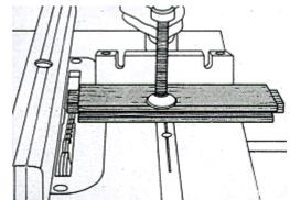
**STEP 5:** Make a special panel-raising fixture such as one of the two shown here. Click on each picture to see larger view.
