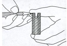
(to make a 1/2" deep cut). Be certain your blade is set to make your cut in the exact center of the stile/rail edge. Make a test cut on a piece of scrap to verify this.
