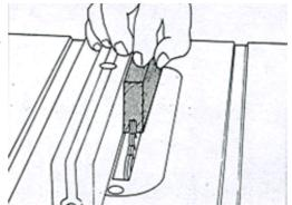
**STEP 2:** Set up your Dado Blade Set to cut the grooves on the insides of your stiles
