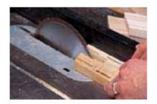
Finger Boards: Cut a 30-degree angle on the end of the board. Cut two parallel, 1/4" slots in the board as shown in the photo. Mark a line 21/2" from the end of the mitre cut. Cut out the 5/8" notches in the sides and then cut out 1/8" fingers with a 1/8" spacing, ripping to the 2-1/2" pencil mark. Stop and back the board out of the cut.
