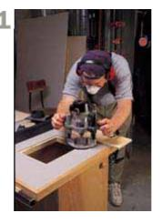
**Routing the Plate Opening:** A good way to get a parallel and square opening is to use the saw fence as a guide for two of the cuts.
