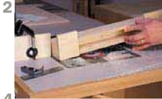
**Routing Slots in the Fence:** Clamp a stop to the saw fence to stop the assembly at the end of its cut. Drill a 1/4" hole at the beginning of the cut and with the router running, lean the fence assembly against the stop, touching the table and lever it down over the hole that you just drilled. Gently push the assembly to the end of its cut and lever-lift the assembly off the table.
