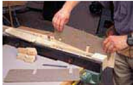
**3 Jointer Insert:** For edge jointing, cut a piece of laminate to the size of one fence face. Make it a little tall so you can pull it out from between the fence face and the fence. Cut two slots to clear the bolts on the fence. Chuck a straight bit in the router and set it flush with the offset fence face and you've made an edge jointer. Pull the spacer out to resume normal operation.
