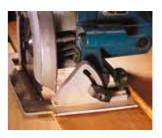
Make the cut with the circular saw motor hanging over the guide – this arrangement provides the most support for the saw and keeps it from tipping.
