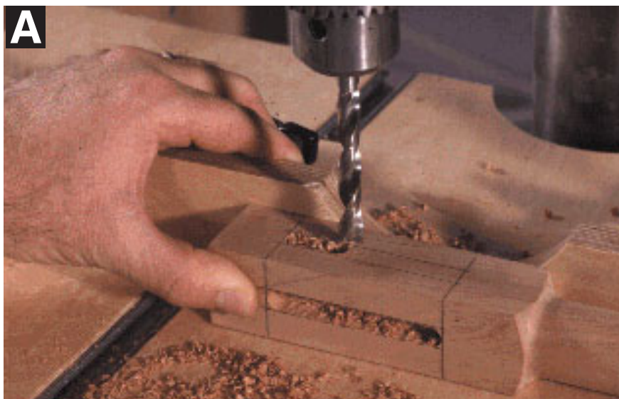
Mark the mortise locations carefully, and use a drill press with a fence for alignment to remove most of the stock.
