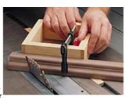
The Jig – To make the jig, cut four pieces of stock for the sides. Rabbet joints at the ends of two of the pieces help align them during glue-up, as shown in the main drawing. (Note: Size the pieces for the box so it clears the blade once it's attached to the runner, as illustrated in the detail at right).
