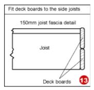
**Step 4:** Finish off your deck by fitting deck boards to the side joists. These serve as a fascia and conceal the ends of the deck boards. For best results the corners of these fascia boards can be mitred.
