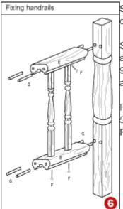
**Step 3:** Measure the distance between the two post positions and cut the top and bottom handrails (**Diagram 6 - E**) to length.
