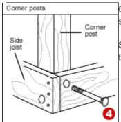
Corner posts will be required at 1200mm intervals on straight sections, fixed directly to the joists of a flat deck.
