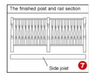
Manoeuvre the finished post and rail section into its position and secure to the joists with bolts.
