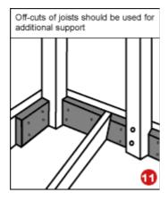
Off-cuts of joists should be used to provide additional support for posts and subsequent decking boards around the posts.
