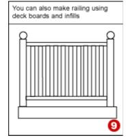
Make sure that the height of the top rail from the finished deck is exactly that of the spindles you have bought, if you don't want to cut them.
