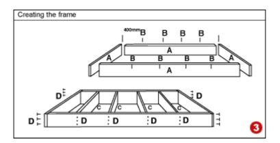
Step 1: Cut the joists (Diagram 3 - A) that will form the sides of the deck to the size you require.
