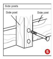
**Step 2:** First mark the position of the posts on the side joists, then bolt the side posts to the inside of the joists.
