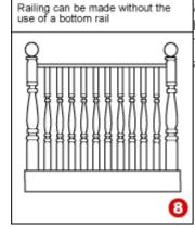
As an alternative, you can create railings without the use of a bottom rail. Posts and top rails are assembled and fixed as before. The spindles are then fixed with screws to the rail and the deck after the deck boards have been fitted.
