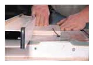
To bevel the crown pieces, first bevel cut one edge (shown) with the table saw blade set at 45°. Then move to your joiner (also set at 45°) and put a ¼" flat at a right angle to your first bevel.
