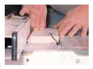
Head back to the saw to cut the second bevel. As you'll see in the photo, by cutting the return bevel on the first edge you've provided a bearing surface for the rip fence, rather than let the bevel slip under the fence, messing up the cut.
