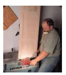
When you trim the doors to size, make sure you support the door adequately and start with the top and bottom edges. That way any tear-out on the end grain and-tenon joinery, and the crown moulding is all simple cuts on the table saw and jointer.
