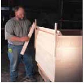
determine if the doors are square by measuring corner to corner. The distance should be the same in both directions. If not, adjust the door by tightening a clamp diagonally across the longer length. When everything is square, tighten the clamps and set the doors aside for the glue to cure.
