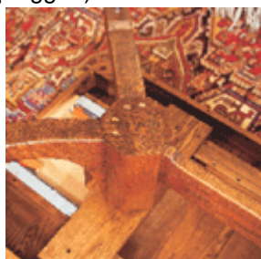
At a joint that needs strength, counterbored screws, glue and #20 biscuits (or dowels) secure the legs to the pedestals
