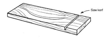
5. Place miter gauge in left table slot and make cross cut through extension.
