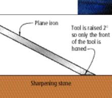
Begin with a 1,000-grit stone and rub the tool back and forth across the work. Try to wear the stone evenly by moving the tool in a regular pattern.
