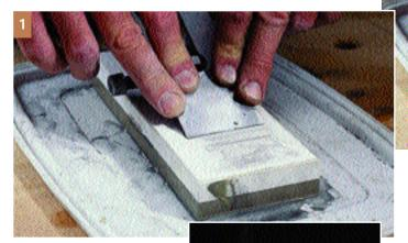
Continue honing the edge by switching to a 4,000-grit stone. Remove the burr on the backside with the 8,000-grit stone.
