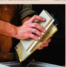
Norton waterstones and the DMT DuoSharp stone are a great combination. The DMT handles the grinding jobs and flattens the Norton waterstones (800-446-1119 or nortonabrasives.com).
