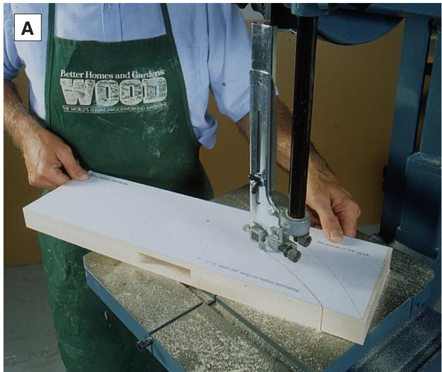
A Adhere the full-size paper pattern to the foot lamination, then bandsaw just outside the marked cutlines to cut the foot to shape.
