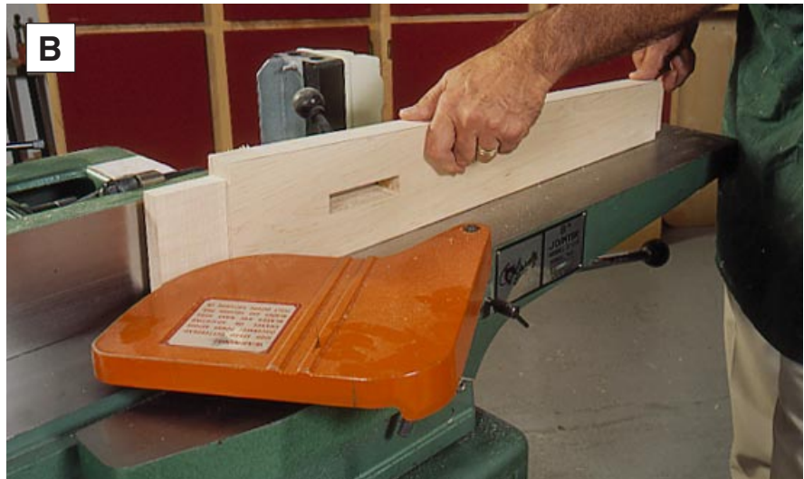
B After cutting just outside the marked taper lines, use your jointer to joint to the line for a flat edge.
