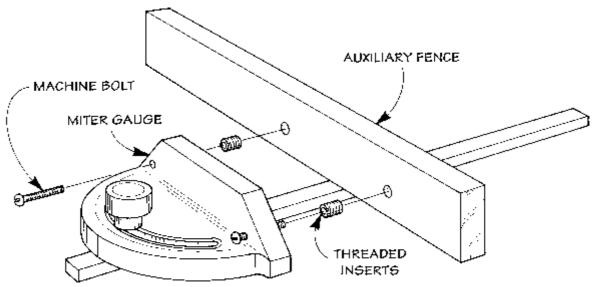
For extra support, I often temporarily screw an auxiliary fence to my mite gauge, see Drawing. The only problem with this is that the woodscrews eventually strip out the holes in the auxiliary fence.
