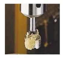
In order to create more room for the chips, I modified bits that clogged by "opening" up the mouth. To do this, file or grind back the top edges of the opening, see drawings.
