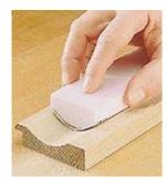
The best sanding block is one that matches the shape to be sanded. So recently when I had to sand some cove molding, I made some custom sanding blocks from 1½"-thick foam insulation.
