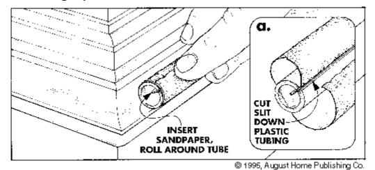
To sand coves, I wrap sandpaper around small lengths of clear flexible plastic tubing. Most hardware stores carry this type of tubing. Choose a diameter smaller than the radius of the cove.
