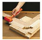
It's a challenge gluing mitre joints. There just isn't an easy way to clamp them together. The store-bought clamps I've tried in the past didn't always pull the joint together. So I came up with a shop-built corner clamp that uses wedges to push (or press) the metered pieces together.
