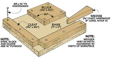
They apply pressure in two directions at the same time. When the inside wedge (the one contacting the metered piece) is tapped forward, it pushes the joint tighter together and firmly holds the piece in place while the glue dries.
