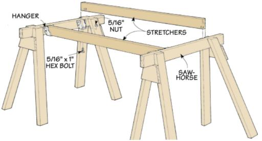
To keep the stretchers from accidentally slipping out of the hangers, they fit onto a metal pin in each hanger. This "locking" pin is just a bolt that passes through a hole drilled in the joist hanger, as shown in the drawing at right. Tightening a nut on the end of each bolt holds it in place. To fit the stretcher over the bolt and nut, all you need to do is drill a pair of counter bores near the end of each stretcher.
