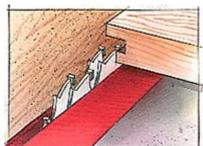
**7.** Raise the dado set for a 3/8"-deep cut. Readjust the fence so the dado set just grazes it. Position your drawer fronts face side up on the saw and complete the cuts on their ends, as shown.
