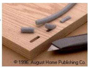
To do this, I plugged each mortise temporarily with foam caulking rod, see photo. The caulking rod I used was slightly wider than the mortises. After the finish dried, I just removed the foam rod.
