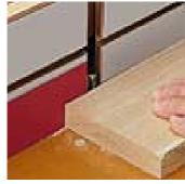
**W**ith just a strip of plastic laminate, you can convert a router table into an edge jointer. In fact, a "router-jointer" puts a surprisingly straight edge on a work piece.
