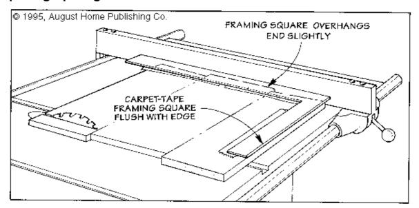
Squaring-up a large glued-up panel on the table saw can be a challenge. Especially if the panel is too large to be supported by the mitre gauge. And the ends of the panel are uneven so you can't run them along the rip fence.
