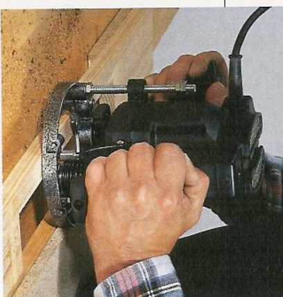
Scrap wood clamped to the workpiece serves as a straightedge guide for the router to follow. This router's base plate has one flat edge to help guide.
