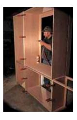
Then use spring clamps at the back to hold everything together as you screw the upper cabinets together and the lower cabinets together. Be sure to screw right behind the face frame so the screw is less visible.
