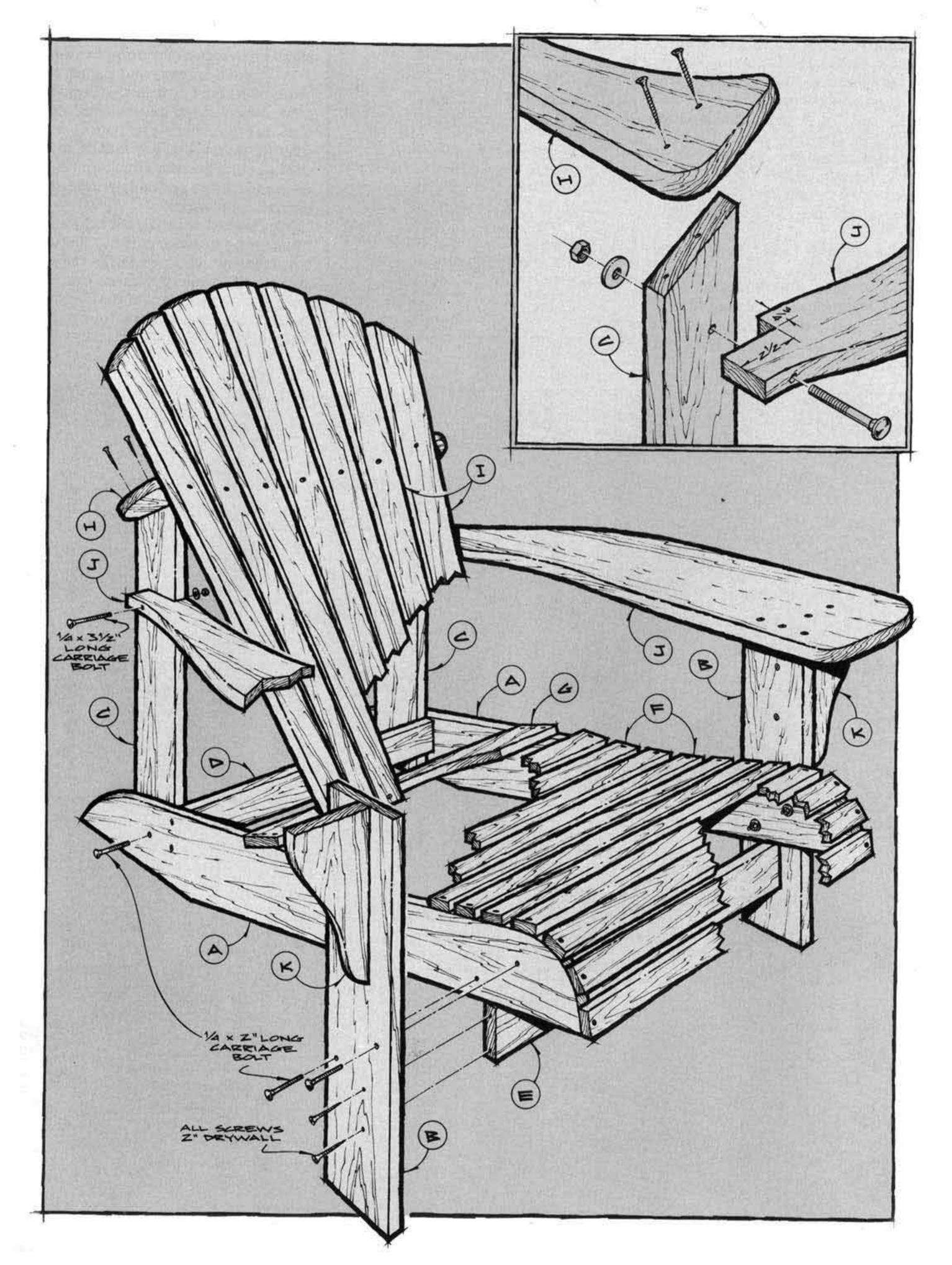
The seven back slats (I) are all cut on the table saw, using a simple tapering jig (described in The Beginning Woodworker column in March/April 1986). All should be cut to the same initial dimensions (2¾ in. wide tapering to 2 in. and 32 in. long). Then butt the back slats together and scribe a 21 in. radius across the top. Secure the slats with clamps and a cleat (to prevent chattering) and cut the 21 in. radius with a saber saw.
