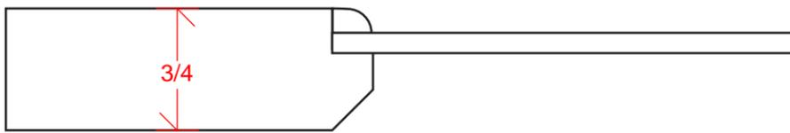
Section through upper door showing glass mounting
