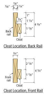
The "X" on the rails and cleats denotes a cross section rather than an end view.
