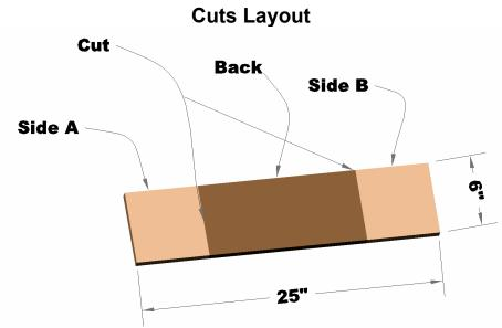
Above shows the cut layout and the amount of stock required to complete the sides and the back piece. The overall piece measures 25" by 6".
