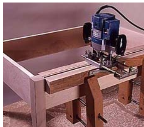
8--Glue and clamp the aprons and legs. Heavy cauls distribute clamping pressure across each apron.
