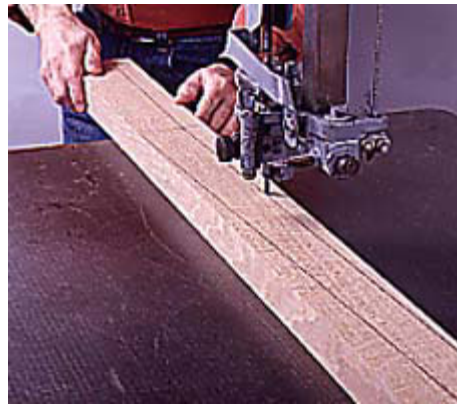
3--Make a template for the shape of the back legs and trace it onto the leg stock. Cut along the outline with a band saw.
