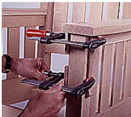
20--Cut the corbel brackets to size and finish sand them. Then glue and clamp them to the outside of the front legs.
