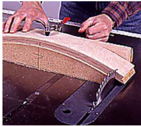
15--Use the inner bending form as a jig for cutting the back rails. Attach the form to a backer board and the saw fence.
