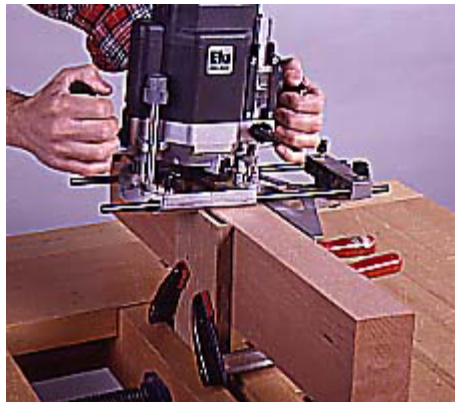
6--Cut the mortises for the loose tenons on the side rails using a router and edge guide. Clamp a block in place for support.
