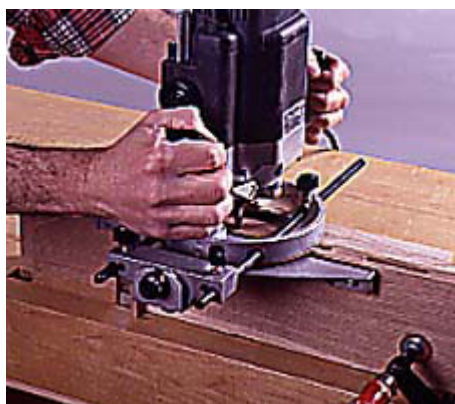
8--Clamp the side rails to the bench to route the mortises for the side slats. Support the router with scrap blocks.
