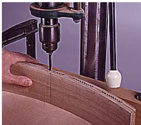
16--Lay out the slat mortises in the back rails, then remove the waste using a drill press. Finish the cut with a sharp chisel.
