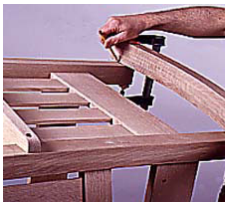
18--Assemble the chair pieces and clamp each rocker over the legs. Trace the proper cutting angle onto the legs.
