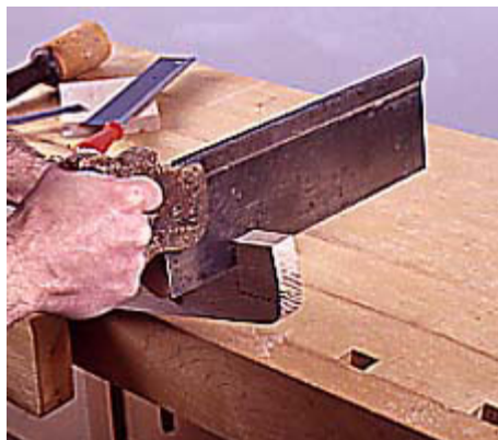
9--Lay out the notch at the back of the arms that fits around the back legs. Using a backsaw, carefully cut out the waste.
