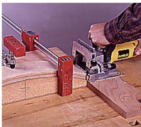
17--Use the bending form to clamp the back rail assemblies to the bench. Then carefully cut plate slots in the rail ends.
