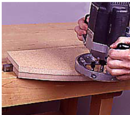
13--Cut the stock for the bending forms to rough size. Then cut it to finish size using the pattern and a flush trimming bit.
