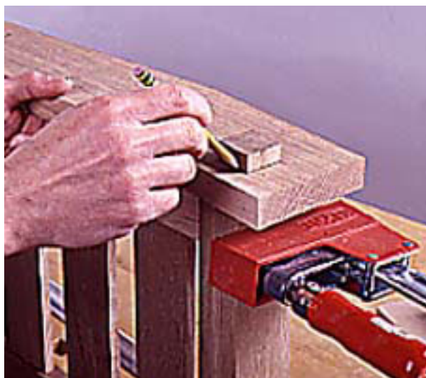
9--Lay out the notch at the back of the arms that fits around the back legs. Using a backsaw, carefully cut out the waste.
