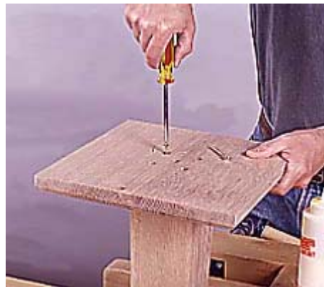
5--Cut the upper base to size and bore a 9/16-in. hole through its centerpoint. Attach it with glue and screws.
