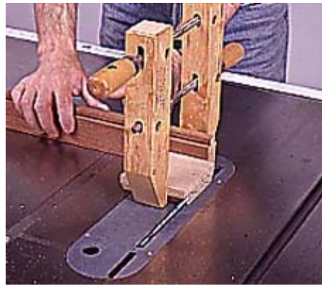
3--Cut the top cap to size, then use a table saw to cut a bevel on the bottom edge. Clamp the block to the miter gauge.
