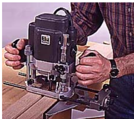
1--Rout a groove down the center for both halves of the lamp post. Use a 5/8-in.-dia. straight bit and a router edge guide.
