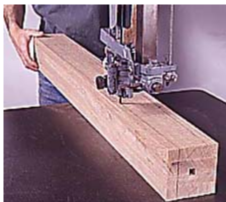
2--Lay out the taper on opposite sides of the post. Then, cut off the waste with a band saw. Mark the other sides and cut them.
