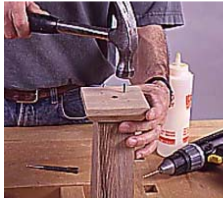
4--Bore a 9/16-in. hole through the top cap, then glue and nail the cap to the top of the post. Bore pilot holes for the nails.
