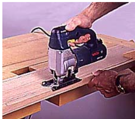
5--Cut the upper base to size and bore a 9/16-in. hole through its centerpoint. Attach it with glue and screws.
